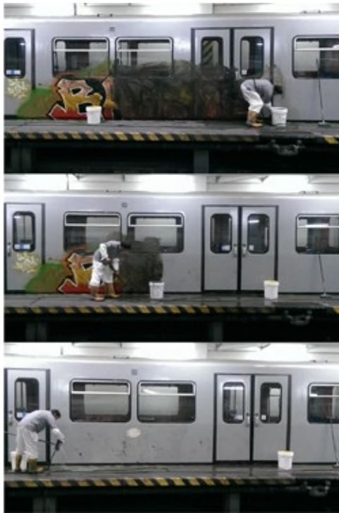
Fig. 2. Cleaning cycle of a metro-train's livery by a contractor Source: Wiener Linien, 2014
