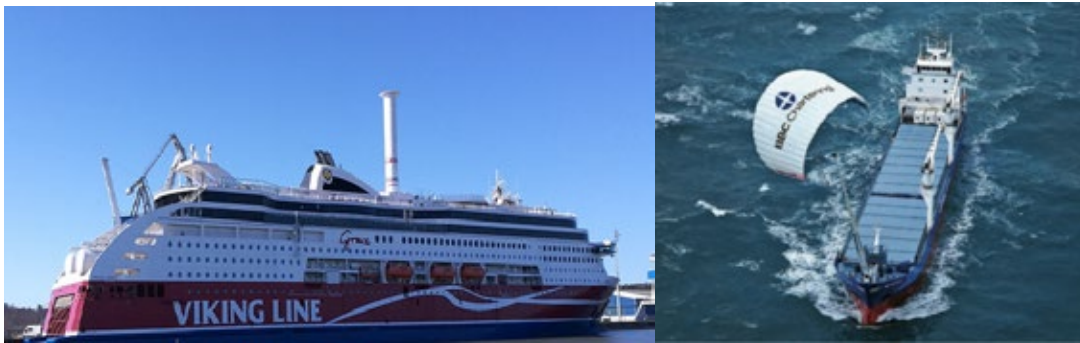
Fig. 2. Flettner rotor on a board of ferry “Viking Grace” and SkySail Source: Norsepower (2018) and SkySail (n.d.)
