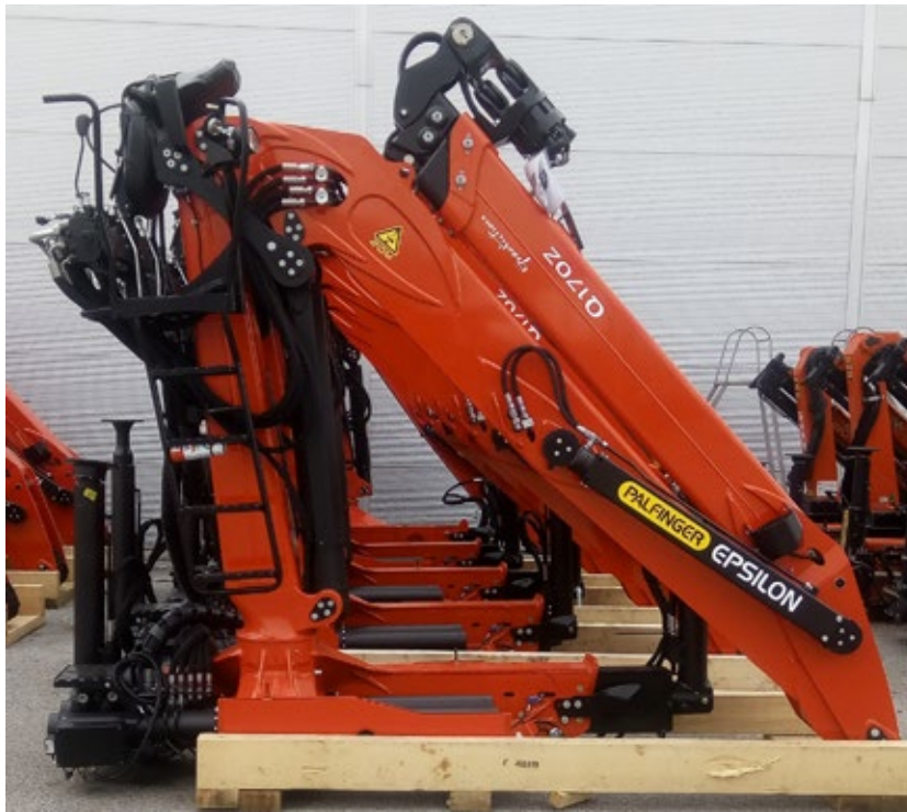
Fig. 3. Hydraulic lifting device PK_6501_HP Source: authors
