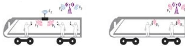
Fig. 2 Access to Internet for Passengers Source: ( www.rosenbergerap.com/Solutions )
