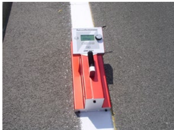
Fig. 1. Device for measuring retroreflection of road markings
