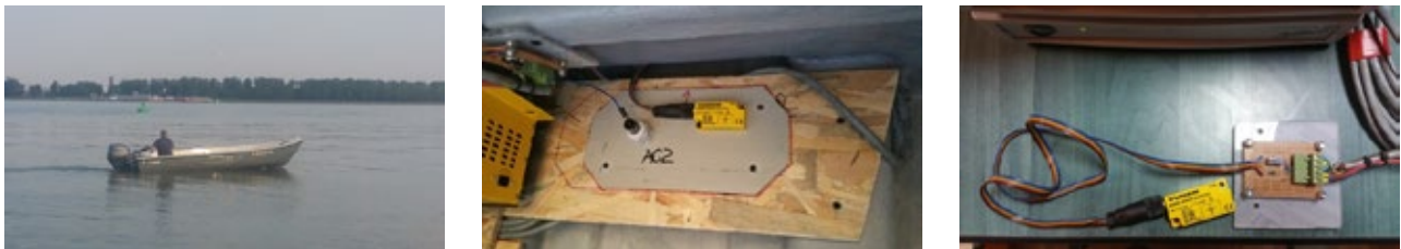
Fig. 6. Experimental trials conducted with full scale model. The installation of the inclinometer in the bilge (middle) and the electronic circuit built for the data acquisition (right)
