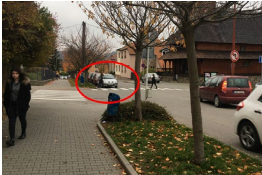
Fig. 5. Insufficient sight distance at the pedestrian crossings Source: authors
