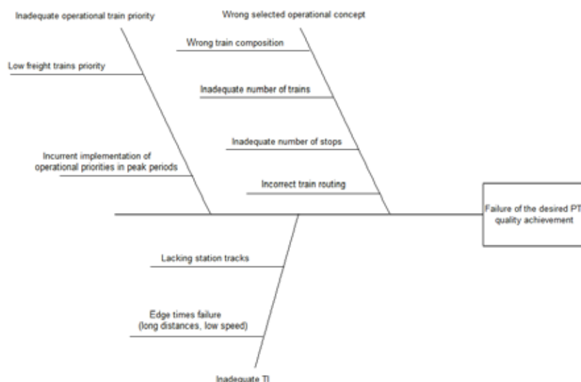
Fig. 1. The Ishikawa Diagram of Failure of the Desired PTT Quality Achievement Source: Authors
