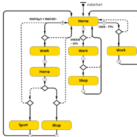
Fig. 3. Diagram of possible scenarios for Employee Agents in AnyLogic Source: own scheme
