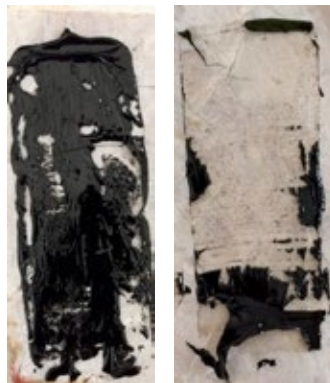
Fig. 5. Peel test results: dry smooth (left), wet smooth (right) limestone samples
